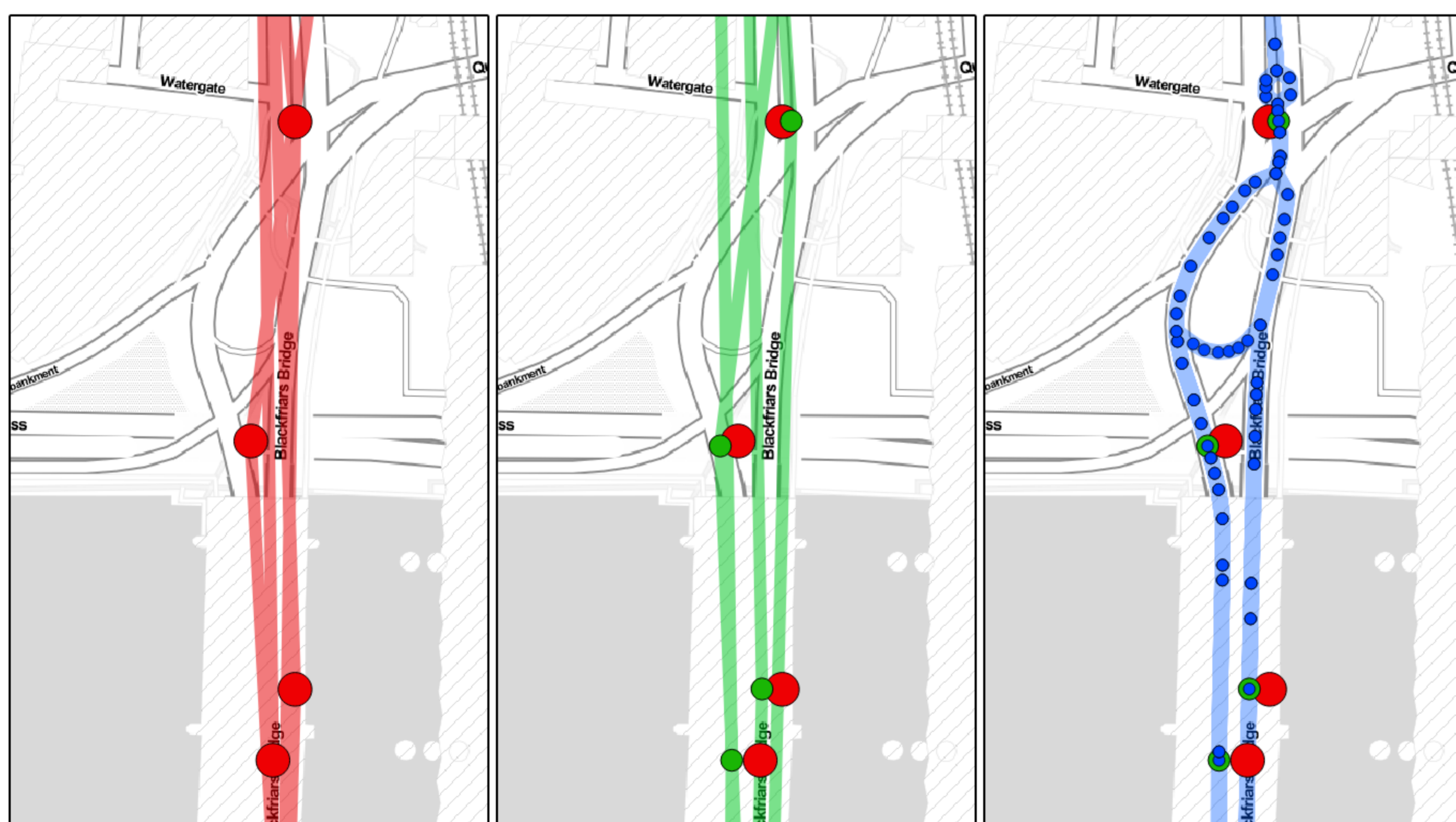
Map matching. Left: Raw waypoint data. Middle: Waypoints snapped to the street network. Right: Interpolation between known visited points, to reconstruct the full path.
